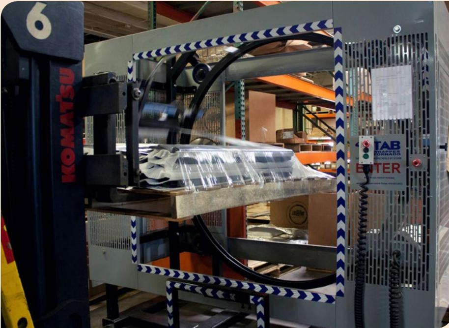
*The TAB Wrapper Tornado encases the entire palletized load in multiple layers of plastic film to keep everything intact and in one place to ensure each order arrives safely and without defects. At DeWys Manufacturing, this TAB Wrapper has replaced wrapping with a horizontal turntable wrapper and by hand.*
