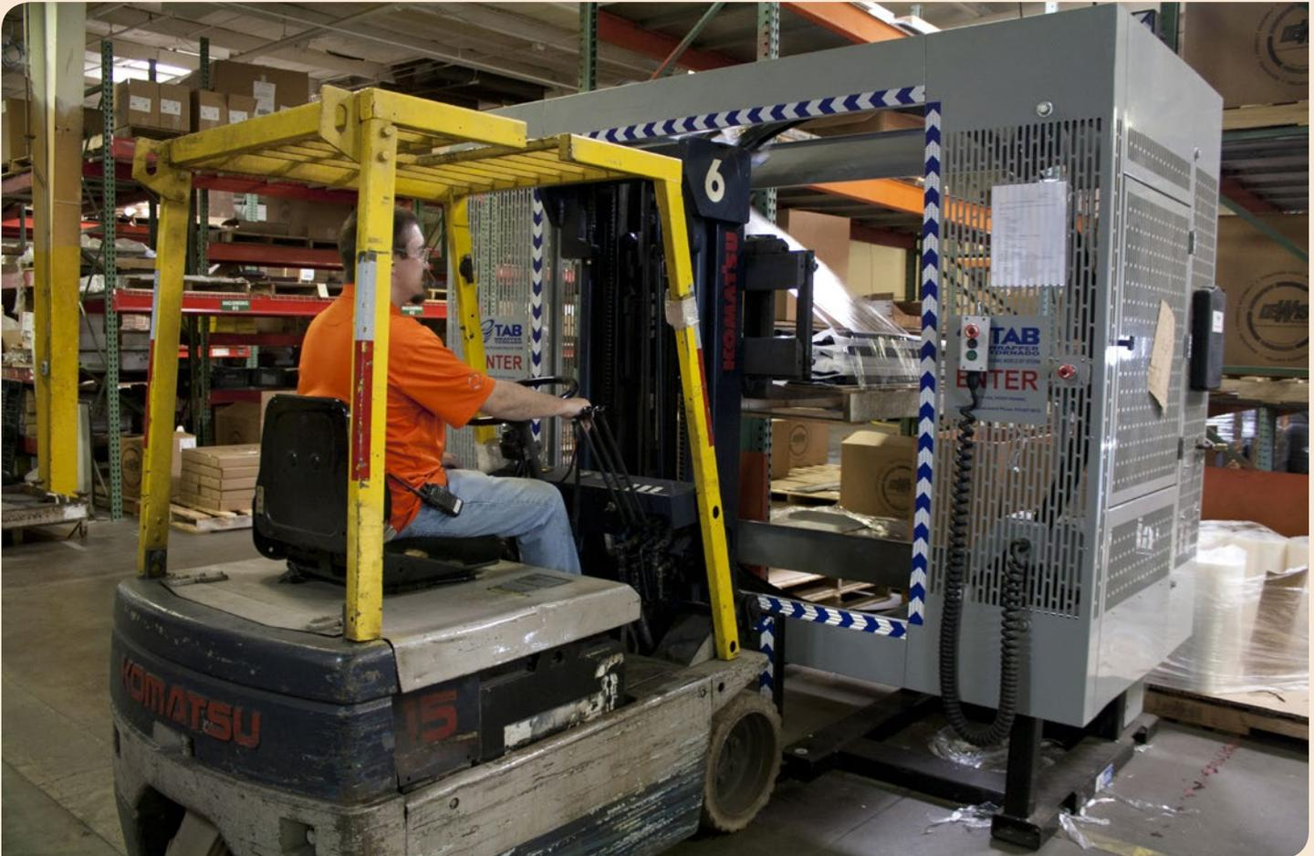
*At DeWys Manufacturing, Marne, Michigan, a lift truck operator wraps a load of metal bars to its pallet using the TAB Wrapper Tornado orbital wrapping machine. The TAB Wrapper has stopped the company's palletized loads from shifting during transit, cut the reject rate in half and saved more than 1,000 man-hours of time in packaging.*
