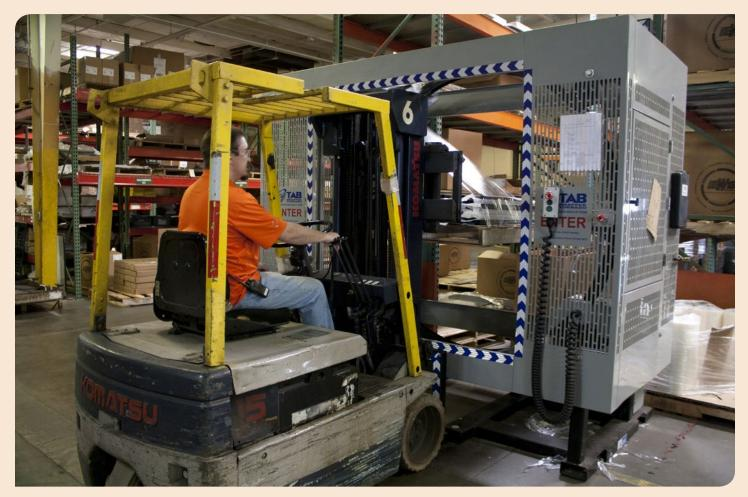
At DeWys Manufacturing, Marne, Michigan, a lift truck operator wraps a load of metal bars to its pallet using the TAB Wrapper Tornado orbital wrapping machine. The TAB Wrapper has stopped the company's palletized loads from shifting during transit, cut the reject rate in half and saved more than 1,000 man-hours of time in packaging.
