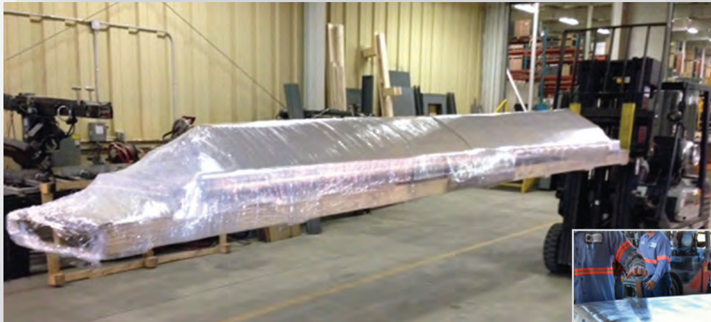
For rods, bars, profiles and other other long products, the TAB Wrapper Tornado can wrap products of virtually unlimited lengths.
